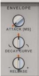
Radical Piano features a special type of envelope generator which is used for shaping the character of the piano sound.
