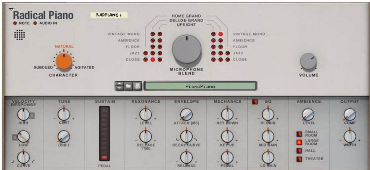
Radical Piano is a Propellerhead Rack Extension device designed to be a straightforward, awesome sounding and very flexible piano. Radical Piano combines sample playback technology with physical modelling to give you great sound quality and seamless dynamic response as well as great freedom to tweak your sounds.
