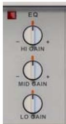
The built-in equalizer is a powerful 3-band EQ with gain controls for the Low, Mid and High bands. The EQ characteristics have been fine tuned and optimized for piano sounds. The gain range is +/-18dB for each of the bands, which makes it easy to quickly achieve great sonic results.
